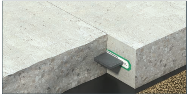
Step 6 Once plates have been correctly positioned, install the specified reinforcement and carry out the next pour. (For expansion joints, install compressible material before second pour)
