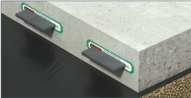
Step 5 Firmly place the Biscuit Plate Dowel into the insertion hole in the sleeve by punching through the sticker as shown above.
