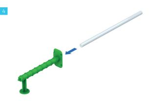
Insert dowels into the Universal Dowel Sleeves by pressing all the way to the end of the sleeve.
