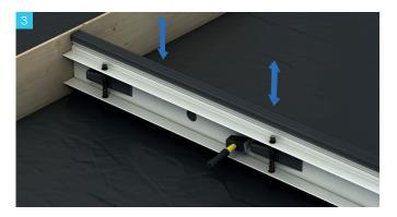
Adjust the profile to the correct height and secure by tapping in the supplied wedges.
