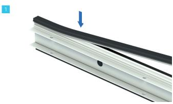
In the case where permanent capping or a rebate mould is used, ensure it is pushed firmly onto the top of the system prior to placement.
