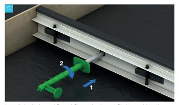
Install the Universal Dowel Sleeve in the profile by pushing the dowel through the foam at the centre of the pre-punched holes and twist the sleeve 90 degrees to fix in place.
