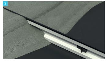
Place the reinforcement and pour the concrete over the key joint. Finish concrete surface to the to of the joint (**not below it**). Always pour concrete evenly to both sides of the joint and ensure concrete is compacted into the keyways.
