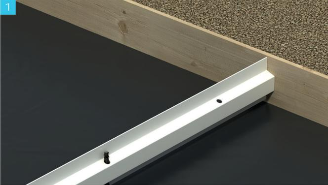
Point key joint in desired location and drive in the supplied pegs. Note that the **longest flange** of the key joint always goes **to the top**.
