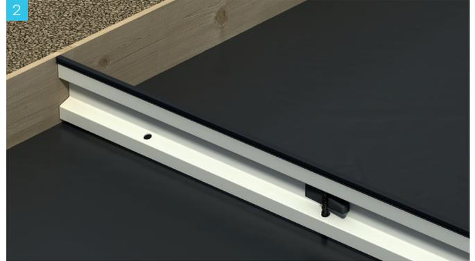
Adjust the key joint to the correct height and secure by tapping in the supplied wedges. If capping strips are to be used allow the appropriate set down distance and ally capping strip prior to pouring concrete.
