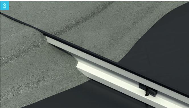
Place the reinforcement and pour the concrete over the key joint. Finish concrete surface to the top of the joint (**not below it**). Always pour concrete evenly to both sides of the joint and ensure concrete is compacted into the keyways.
